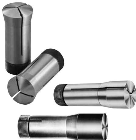
Even with the best of planning, emergencies arise when your tool room and production departments require a stepped, odd size or special-shape collet. On such occasions, use the Hardinge® **Emergency Collet**. The soft face and pilot hole permit rapid drilling, boring or stepping out to the exact size required. Pins are supplied for precision machining. Emergency collets have internal threads for positive stops.
