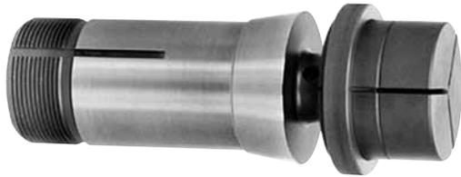
The Hardinge® Super-Precision® **Master Expanding Collet** is a valuable aid for close tolerance machining. There is no end movement of the master expanding collet or pads. The collet threads are separate from the collet body and pull back to operate the expander. The shoulder on the machineable pads locates the work for Dead-Length® control for facing repetitive parts to the same length. No spindle nose cap is required.
