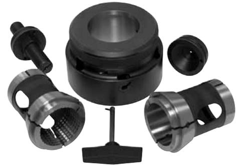
These units can be used for Dead-Length applications on lathes with A2-6 spindle noses. Separate link-ups will be needed for other lathes. Collet sold separately.
