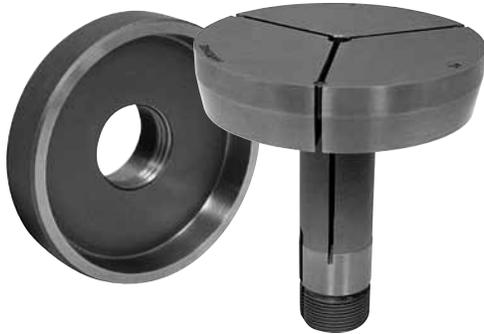
Emergency step chucks are made of soft, machineable steel, while closers are made of cast iron. Step chucks with small closing angles are available for use in stationary (non-rotating) workholding devices. Contact us for more information.
