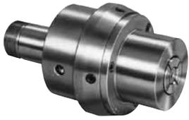
The Model-S Expanding collet draw plug expands at the front of the collet, resulting in maximum gripping force in the bore of a small diameter workpiece. For larger diameter workpieces, Hardinge recommends the Sure-Grip® Expanding Collet System.
