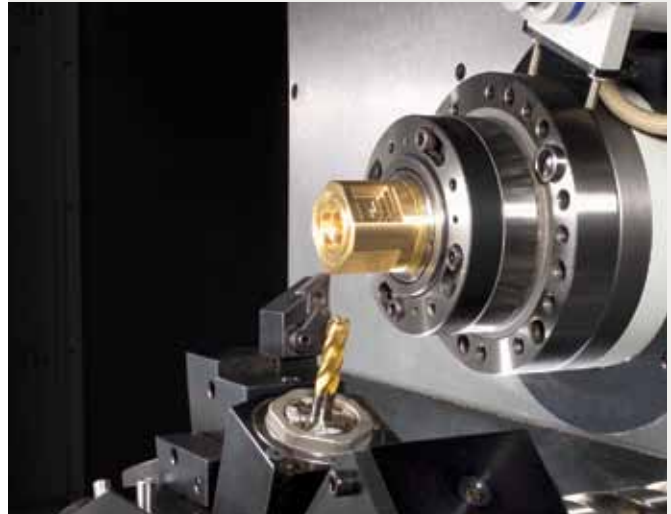
Cover Photo: B42 Collet application on a Hardinge QUEST ® LMC42 Lean Manufacturing Center
