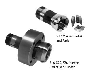
The **Style "S" Master Collet**, although originally designed for first operation machining on multi-spindle automatic screw machines, has many benefits to the CNC lathe operator. The collet pads can be changed much quicker than a standard solid collet, the cost is less and it requires much less storage space. Depending on size, the TIR for the master collet and pads is .004" to .008".
