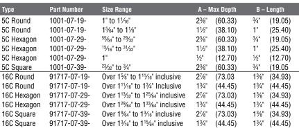
NOTE: Millimeters in parentheses, 5C-SC step collets have internal stop threads. Part numbers preceded by 9 are special order:
