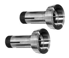
Step Chucks are used for accurately holding work up to 6" in diameter. Castings, moldings, stampings and machined parts are held rigidly and accurately. Tubing can be held without crushing or distorting. Accurate gripping, the same as with collets, is yours when you use regular- and extra-depth capacity step chucks for holding larger diameters.
