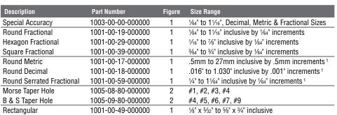
**NOTE:** Round 5C collets above 6%4", hex collets 5%4" and above, square 5C collets 2%2" and over, 5C number collets and letter collets do not have internal threads. For internal threads, see 5C-SC step collets.
