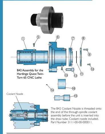
The B42 Stationary Collet Adapter Assembly is a Dead-Length® system designed to provide precise length control of the workpiece. This feature makes it possible to accurately transfer parts from one spindle to the other within .0005" (.0127 mm). The system uses either B42 Solid or B42 Style S10 Master Collets and pads. The B42 Stationary Collet can be used on the Hardinge machines indicated below as well as other machines with an A2-6 spindle nose. Separate linkups will be required.
