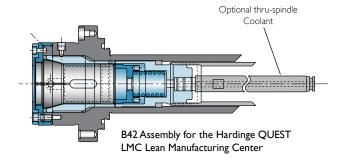
B42 extended-nose collets, expanding collets, ejector stops, chip control and thruspindle coolant are available per application.
