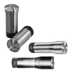
Even with the best of planning, emergencies arise when your tool room and production departments require a stepped, odd size or special-shape collet. On such occasions, use the Hardinge® Emergency Collet. The soft face and pilot hole permit rapid drilling, boring or stepping out to the exact size required. Pins are supplied for precision machining. Emergency collets have internal threads for positive stops.
