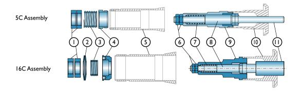
The **Dead-Length Spider-Stop Step Chuck** is designed to handle workpieces larger than the capacity of the Dead-Length 16C Collet or Step Chuck. The spider stop slides through oversize slots in the step chuck and locates against the collet seat in the machine's 16C spindle. A stop button screws into the spider stop and can be machined to locate against the reference location on the workpiece. This system requires a standard extra-depth step chuck closer:
