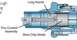
**NOTE:** The chip shield can be installed in all solid and master collets below 2.43" (61.7mm) round.
